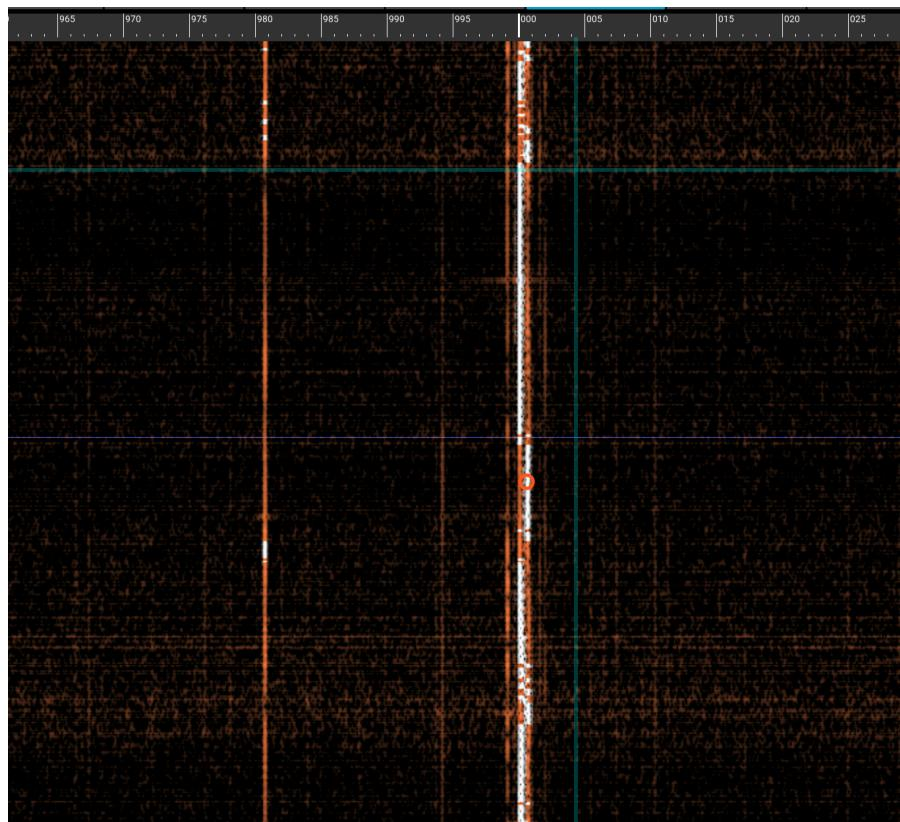
Now across the top of the screen the units are Hz. 000 in the middle represents exactly 1206kHz, then either side of that is the offset in Hz from the centre frequency. So now we can see that there are actually 5 or 6 carriers on the frequency, far beyond our initial thought that we'd find an empty piece of band there.
