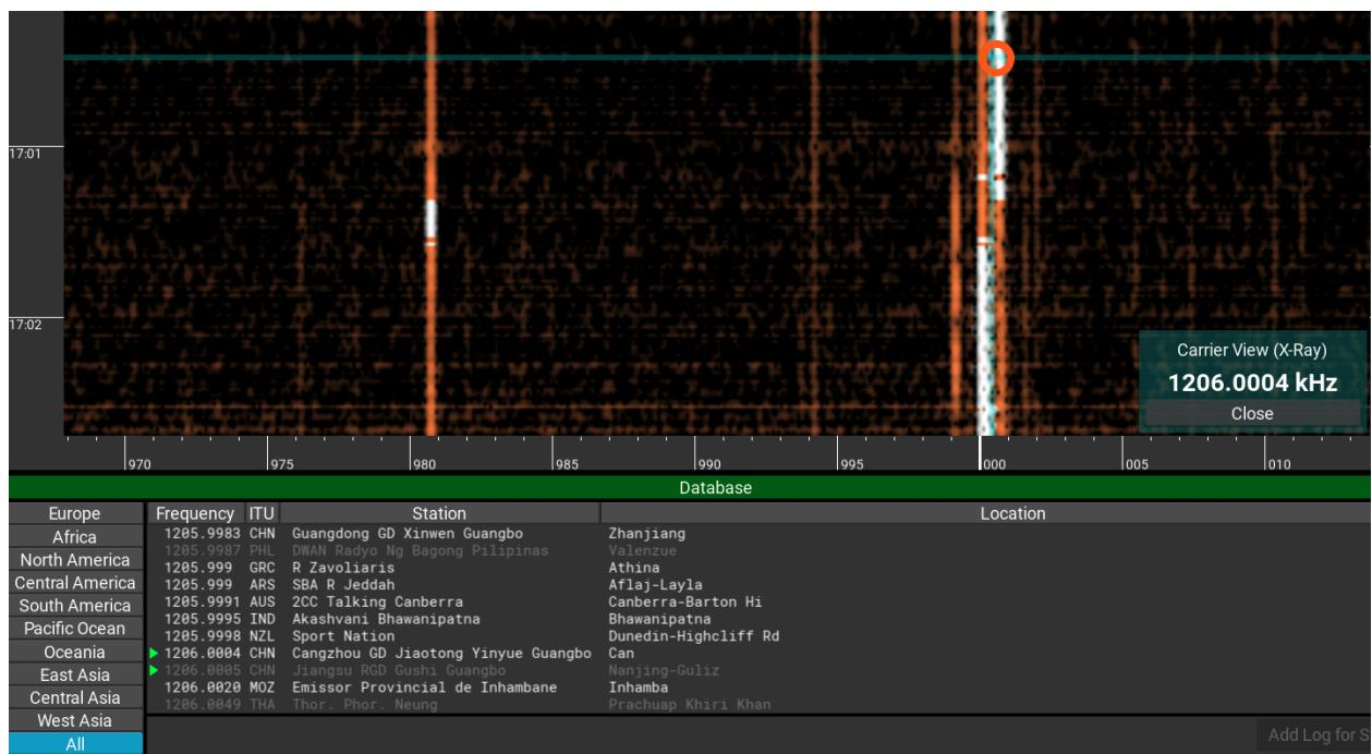
Now at the bottom of the screen you can see a number of stations on 1206kHz, and a small green arrow indicating a match between the carrier that I've clicked on, and stations known to be on that precise frequency. In this case, the carrier could belong to Cangzhou GD Jiaotong Yinyue Guanbo from China. In this example the carrier was so weak that I actually had no audio so identification
